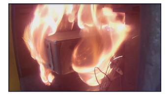
A cell experiencing thermal runaway will rapidly increase in temperature, typically achieving surface temperatures of 400-800°C within seconds of the triggering event. Additionally, gas pressure building within the compromised cell will result in rupture of the cell-wall or, in the case of cylindrical cells, escape through the safety vents located at the positive terminal. Both modes of this venting behavior pose thermal and mechanical dangers to nearby components.
